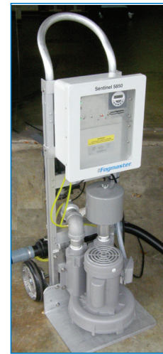
Cart mount unit with 1 hp blower, 2 hose/nozzle assembly, NEMA 4X enclosure, see-thru cover with lockable catches, environmental cable connectors.
